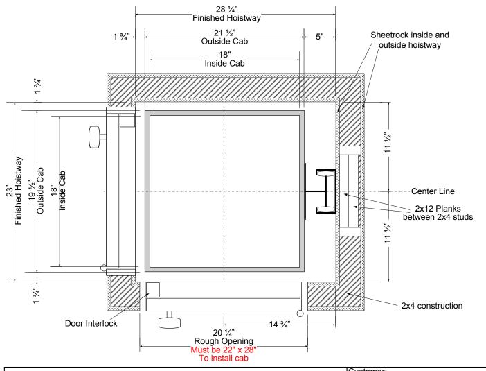
HOISTWAY: The hoistway must be in accordance with "Safety Code for Elevators and Escalators" (ASME A17.1) and all state and local codes.
